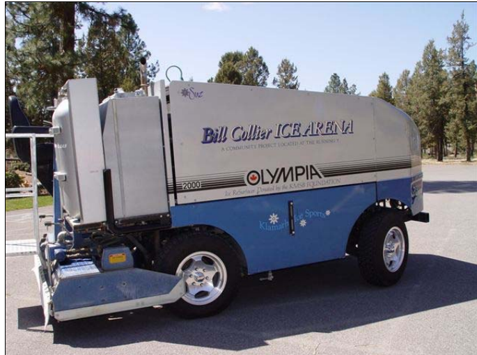
The Suz at The Bill Collier Ice Arena in Klamath Falls is powered by natural gas
