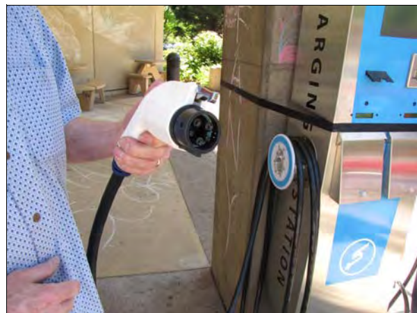
Patrick Box of REDCloud holds the J1772 connector. SOU staff will charge the Ford Ranger by connecting the J1772 to the charging station set up at the public works shop. However if they drive to a location that does not have a charging station, they can plug the Ranger into a standard household outlet (120 volts).
