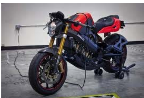
The Empulse on-board charger can be plugged into a standard outlet.
